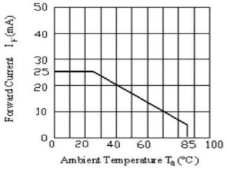
For operation above 25 °C,The lfm & Pd must be derated , the current derating is -0.36mA/ °C for DC drive and -0.86mA/ °C for Pulse drive ,the Power dissipation is -0.75mW/ °C.The product working current must not more than the 60% of the lfm or lfp according to the working temperature.
